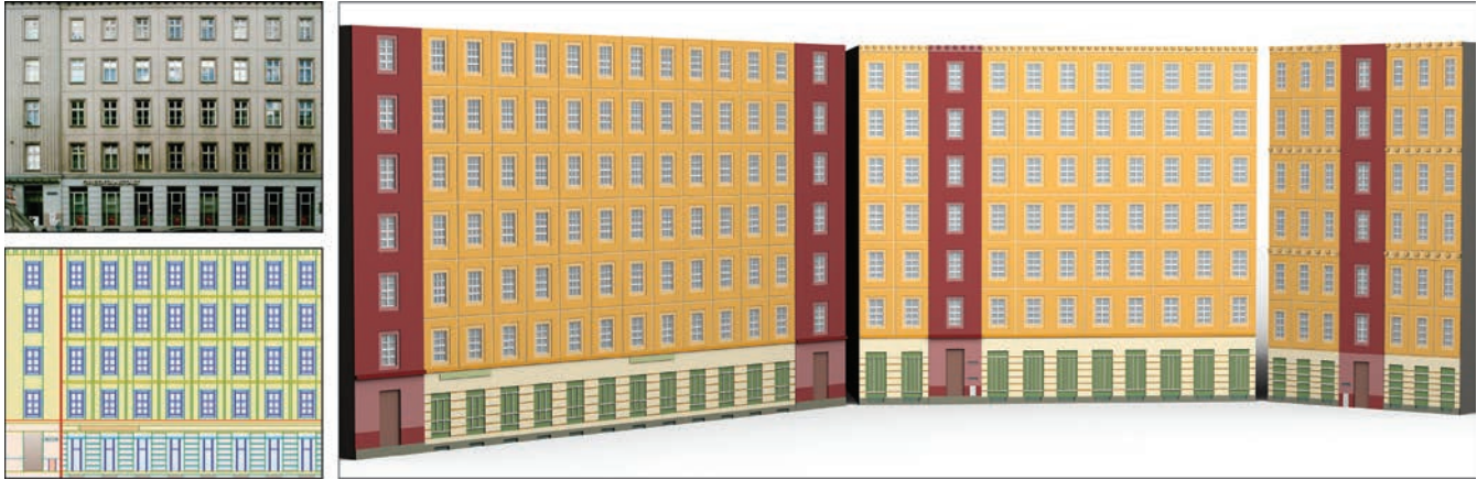
Fig. 9. Example facade (taken from Müller et al. [2007]; top left) with its hierarchical segmentation (bottom left) and three layout variations (right). The modeled constraints enforce the alignment of windows and doors in the columns and floors of this design, even though the ornamental row can be optionally repeated between floors. The relayouting algorithm also finds creative new layouts for the panels of the door-sized windows in the first floor in all three examples. The shuffling of elements enables the door column to appear multiple times and to occur in different positions. The sign on the first floor and the other ornaments can break the translational symmetry of the columns.
